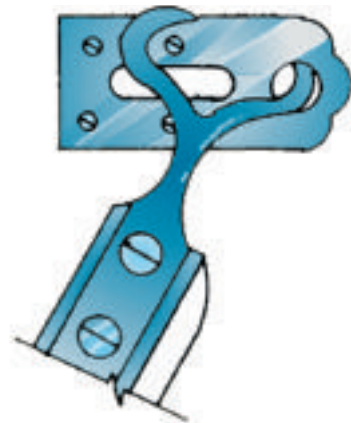
STAGE BRACE CLEAT W/ BRACE HOOKED
