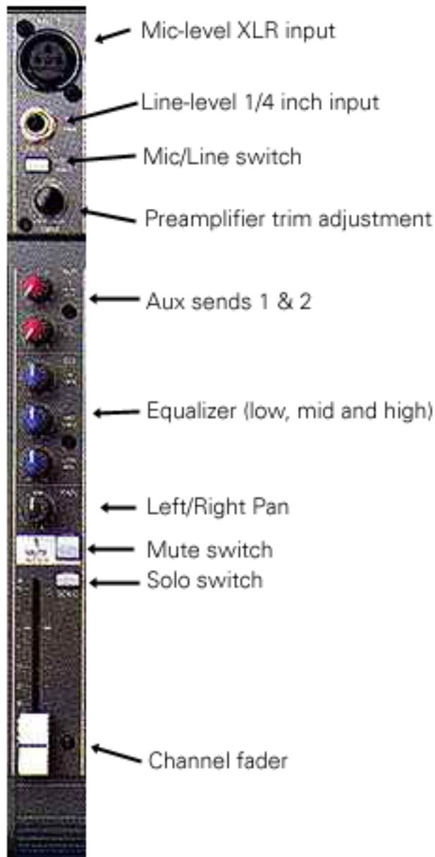
Figure 6.5: The typical elements of an input channel on a mixer. This is representative of a relatively small mixer. Larger boards usually have a larger equalization section, more aux sends, and output channel assignment switches.
