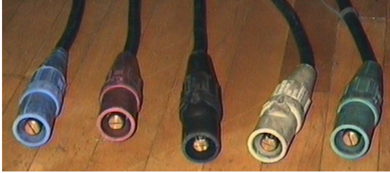
Figure 7.2: Cam-Lok power connectors, often used to connect equipment to a venue’s power feed. Cam-loks can carry very large amounts of current and provide a locking mechanism so the connectors will not come apart under normal conditions. Note the color-coded boots, used to differentiate between ground (green), neutral (white), and the three hot phases (black, red, blue).
