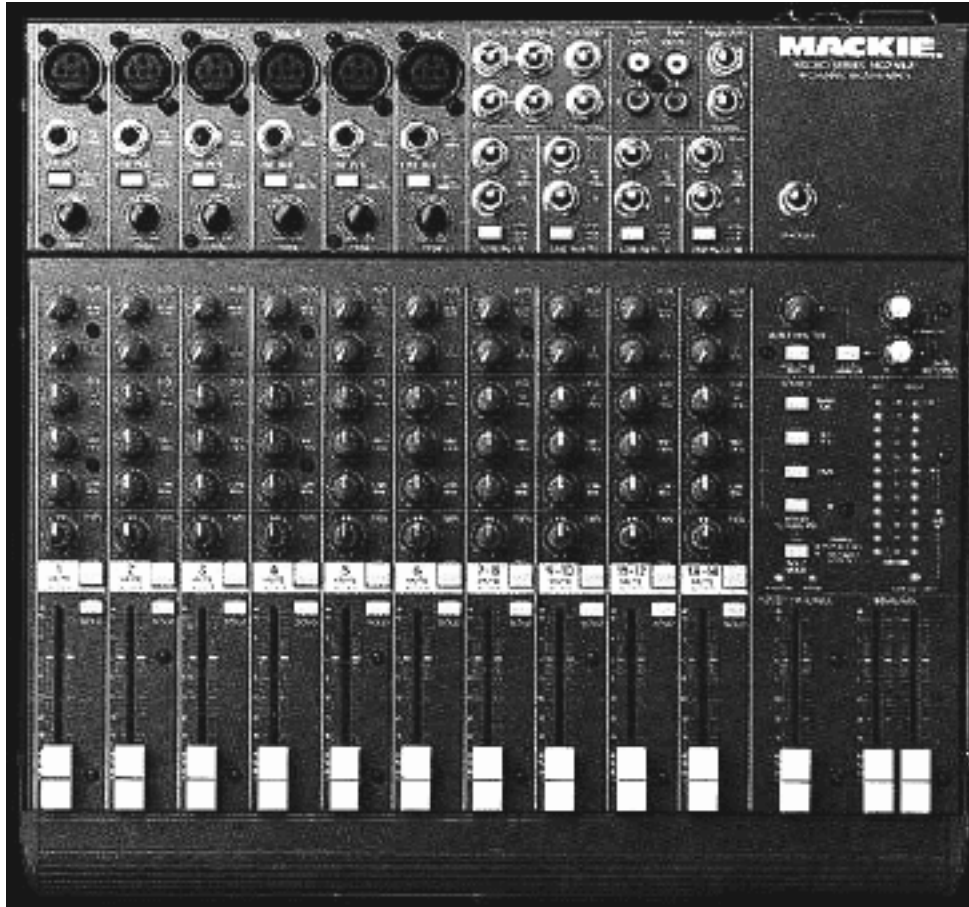
Figure 6.4: A 14-input mixing board, manufactured by Mackie Designs, Inc. Small boards such as this offer plenty of capability for most theatre shows, and should be used in place of large boards where possible.
