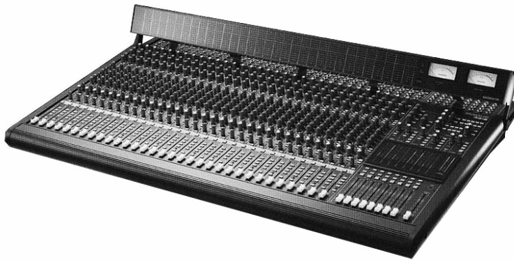
Figure 6.6: A 32-input mixing board with eight discrete output buses, manufactured by Mackie Designs, Inc. This particular model of mixer is owned by WPI, and is often used for large theatre shows.
