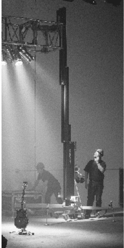
Figure 4.7: A Genie Industries SuperTower being used to hold lighting truss.
