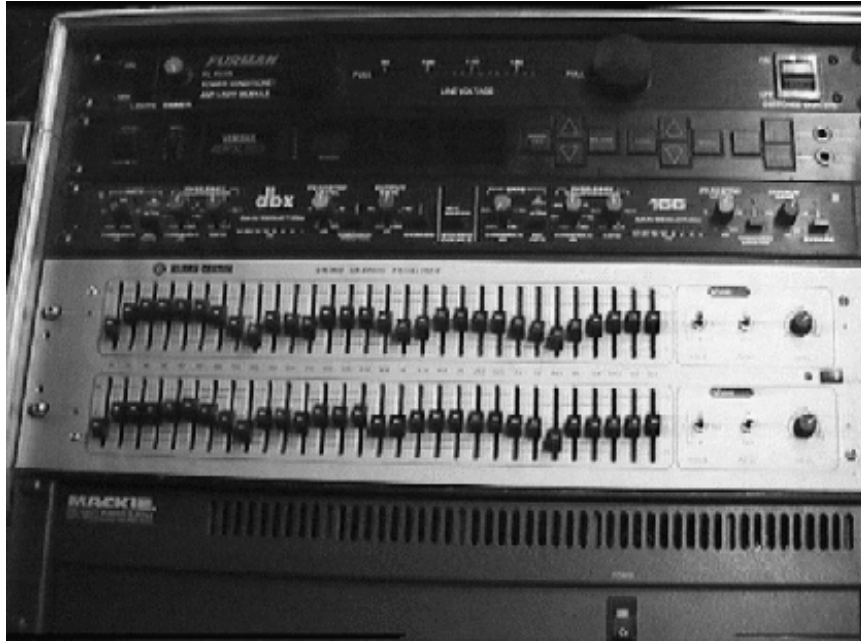
Figure 6.8: A roadcase with several pieces of signal processing equipment, including a dbx compressor/limiter, a Yamaha effects processor, and a Klark-Techne graphic equalizer.
