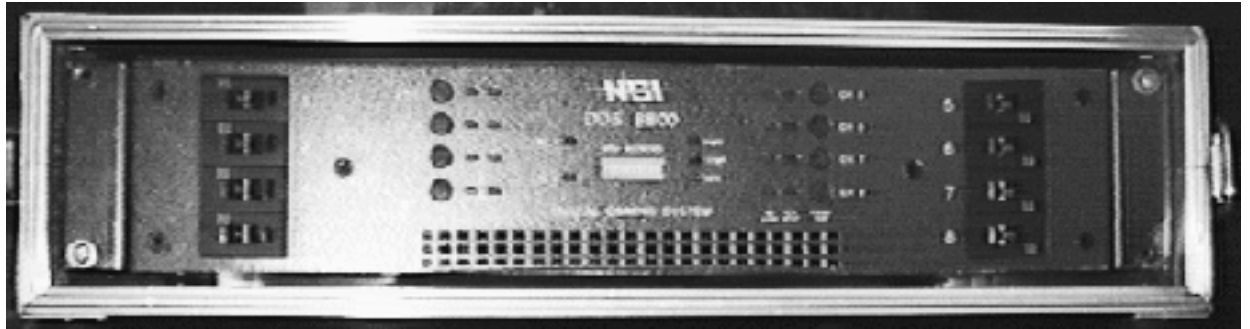
Figure 5.17: The front panel of a digitally controlled dimmer, manufactured by NSI, Inc. Dimmers such as these are often used at WPI to control a variety of small lighting instruments such as PAR 16's, practicals, etc.
