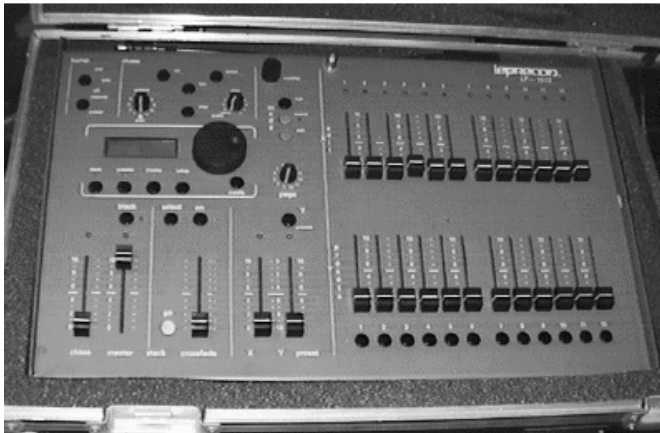
Figure 5.19: Small but powerful lighting board, manufactured by Leprecon/CAE, Inc. This board is used to run the lights in many of the small productions at WPI.
