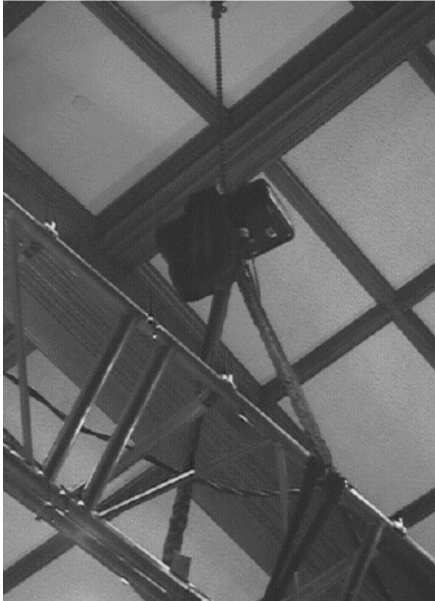
Figure 4.9: A CM Lodestar chain motor with slings and lighting truss, flown from the ceiling in Alden Hall at WPI.
