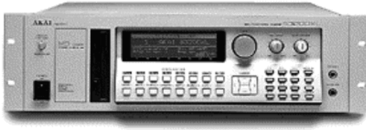
Figure 6.3: An advanced digital audio sampler, manufactured by Akai . Samplers such as this can store many minutes of audio on an internal hard disk and play it back from a MIDI keyboard or by computer control.
